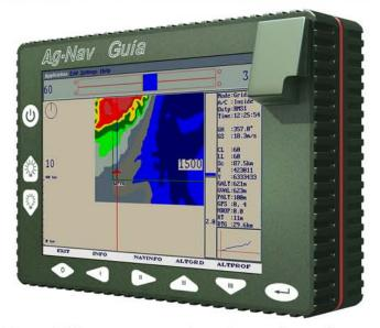
The LiNav is a DGPS navigation system designed to meet the specific requirements for general aerial survey. The LiNav system provides the pilot with swath, directional guidance, and other navigational information required to carry out precise aerial applications.
