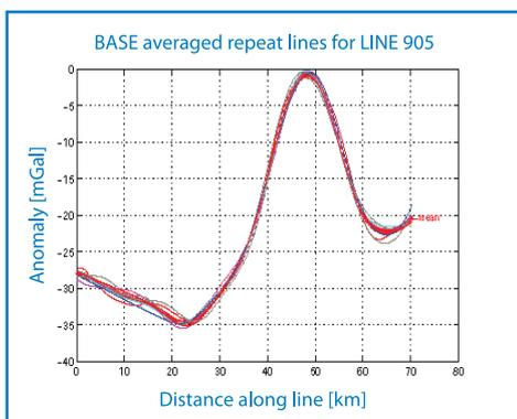
Fig 2. Fixed-wing repeat line RMS Error = 0.5 mGals
